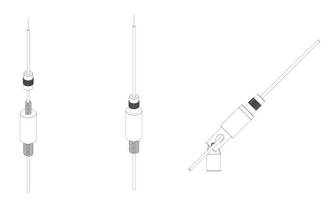
Insert cable into the top of the gripper. Always insert through the plunger at the top unless otherwise stated. Adjust the gripper downwards by pushing the plunger on the top of the gripper.
