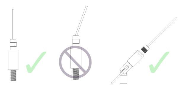
Grippers and ceiling fittings perform best when in a straight line. For angled applications use angle grippers and ceiling fittings. Avoid angled pulls in excess of 5°on straight pull type grippers.
